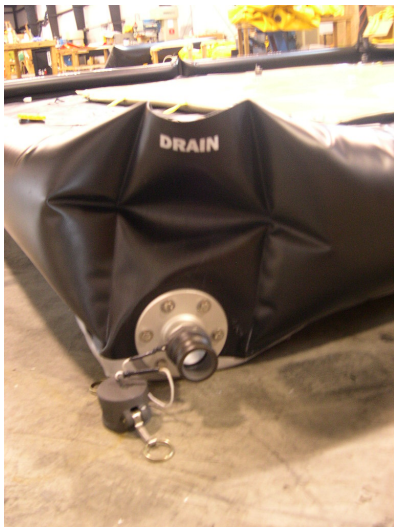
Photo #1: 2”Drain connection
