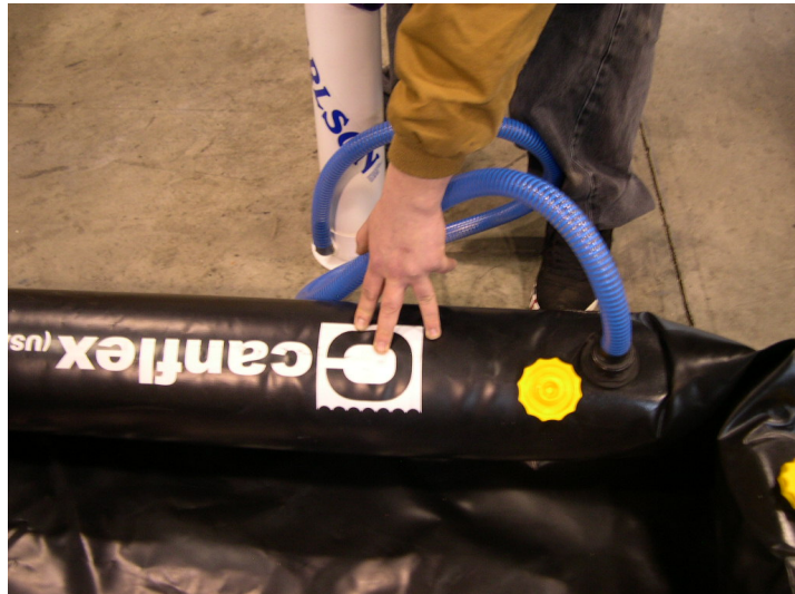
Photo #2: Air tube w/ pump & valves
