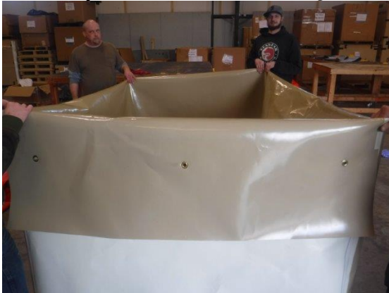
Secondary Containment/ Liner outside Quadcon
