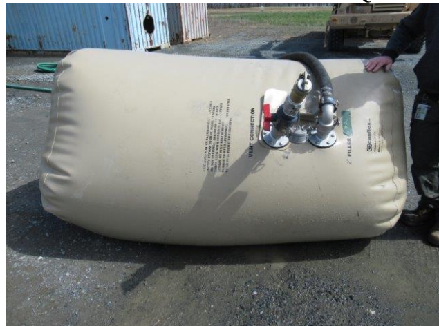
CRT-850 Pressure & Volume Test Outside Quadcon
